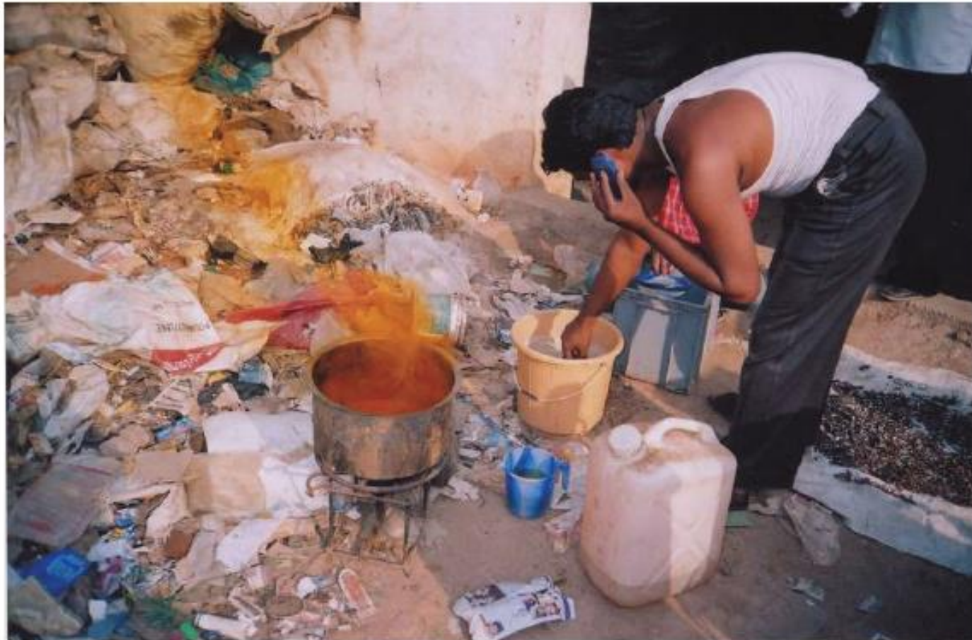
“Low-tech” gold recycling in Bangalore/India (photo by courtesy of EMPA, Switzerland)
